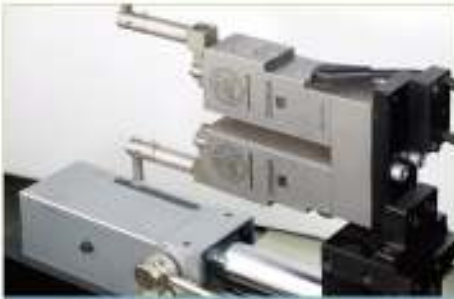
(4) Auto in-process gauge Ø8-90mm Marposs
