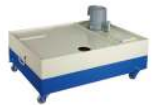
(5) Water pump and tank
