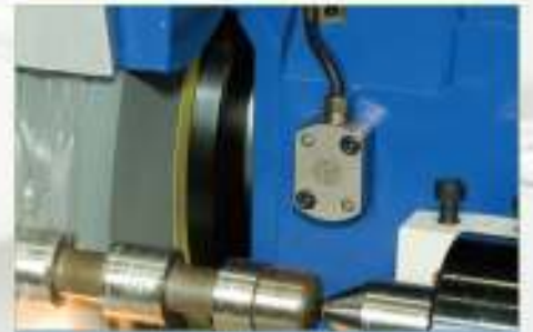
(7) Wheel crash control device Marposs/BS
