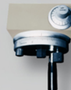
Cross Micrometer Attachment (PSGS) 1 division on cross handwheel: 0.002mm 1 revolution on cross handwheel: 0.04mm
