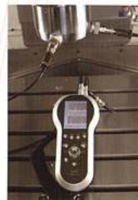
4-channel dynamic signal analyzer. To inspect & analyze spindle vibration and make sure spindle running at perfect conditions.
